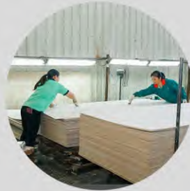
patching of base plywood
