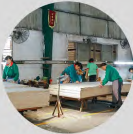
patching of veneered plywood
